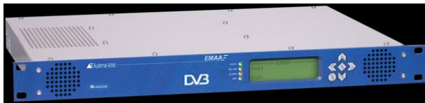
EMAA Transmitter Transmitter MFN / SFN
