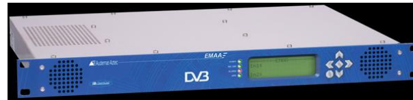
EMAA Zecho Gap filler Iso frequency
